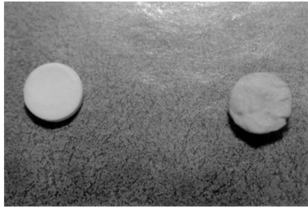
Figure 1 Photograph of examples of the hydroxyapatite disks (HAP) and hydroxyapatite/collagen disks (COHAP) used in this study. The size is 4 mm in diameter, 1 mm in length.
